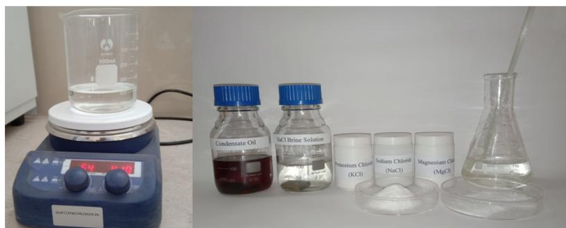
**Figure 3.** Salt stock and brine solutions prepared by blending with a desired amount of salts in distilled water under different temperature conditions.
