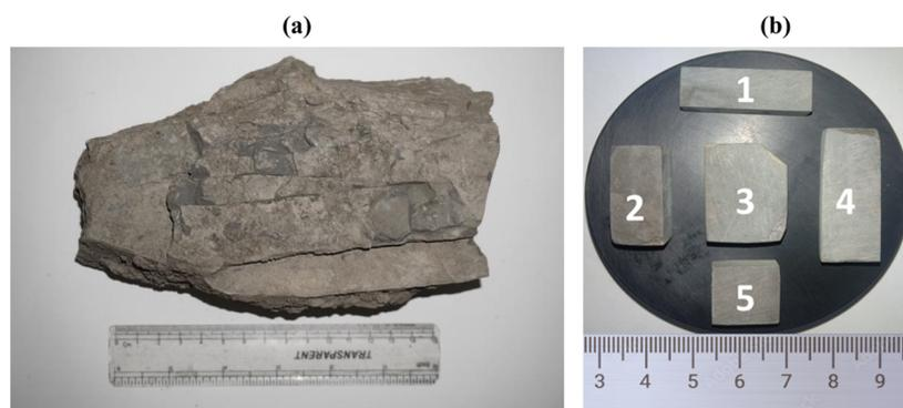
**Figure 2.** Illustration shows the (a) photograph of the shale sample hand specimen and (b) sample prepared for CA measurements.
