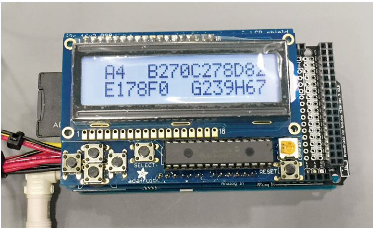
FIGURE 3. Data-logger assembly to record sensor data together with mask temperature and timestamp.
