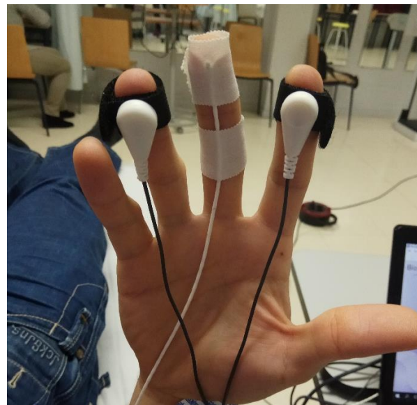
Figure 2. Placement of electrodes for SC and Temp on the right hand.
