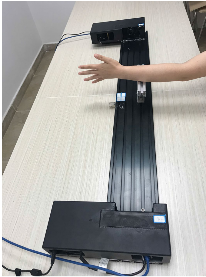
Figure 1. Scanning of actual hand by Gemini structured-light scanning system.
