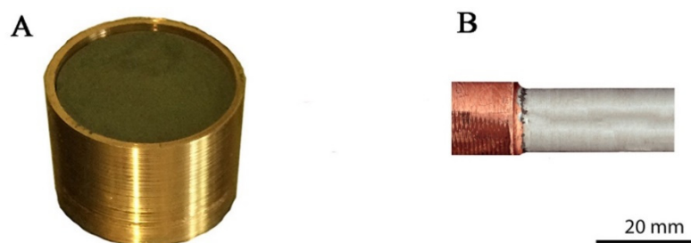
Figure 1. The container with the Zr-Cu mixture before and after the extrusion process: (A) container made of Cu-ETP with the Zr-2.5Cu mixture; (B) product after the extrusion.
