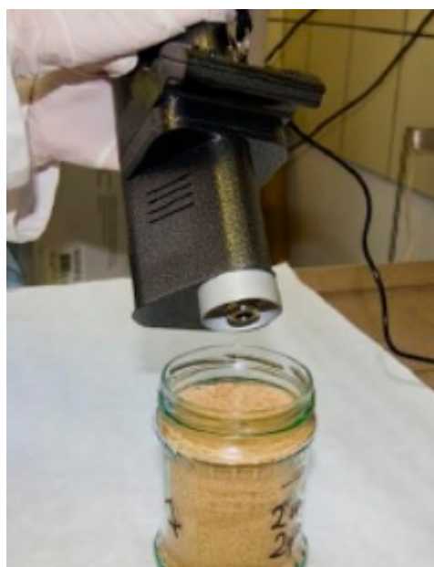
Figure 2. Photo of the sand jar showing the location of the MO-2M detector inlet nozzle.
