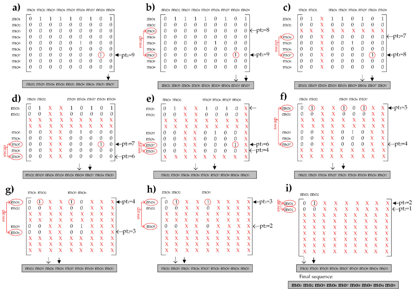
Figure 8. The step-by-step procedure of the constraint handling heuristic: (a) Select the pointer identifying the last machining operation in the sequence, mo 7 ; (b) Swap mo 7 and mo 3 according to the condition in Step 5.II; (c) Exclude row and column of mo 3 , and select the next one, mo 4 ; (d) Swap mo 7 and mo 4 according to the Step 5.II, exclude row and column of mo 4 , and select the next operation, mo 9 ; (e) Swap positions of mo 7 and mo 9 , exclude row and column of mo 9 , and select the next operation, mo 8 ; mo 1 is skipped according to the Step 5.II.f; (f) Swap positions of mo 7 and mo 8 , exclude row and column of mo 8 , and select the next operation, mo 1 ; (g) Swap positions of mo 7 and mo 1 , exclude row and column of mo 7 , and select the next operations, mo 1 and mo 6 ; (h) Leave mo 6 and mo 1 as positioned, exclude row and column of mo 6 , and select the next operation, mo 5 ; (i) mo 1 goes before mo 5 and before the last operation mo 2 ; the final sequence is generated.
