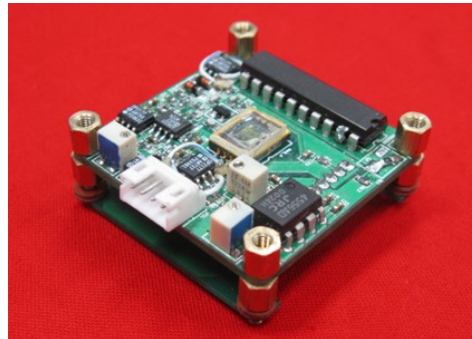
Figure 6. Integrated driving circuit and signal conditioning circuit of the MEMS torsional resonant magnetometer.
