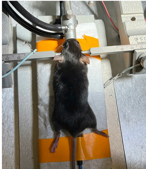
Figure 8. Mouse's head secured centrally with ear bars, in reference to step 62 "Fixation to stereotactic instrument for pump implantation"
