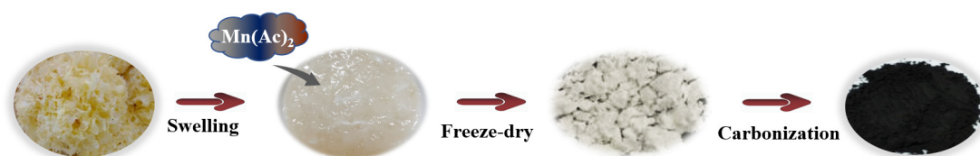
Scheme 2. Schematic illustration of the synthesis of MnO/PC nanohybrid based on the tremella.
