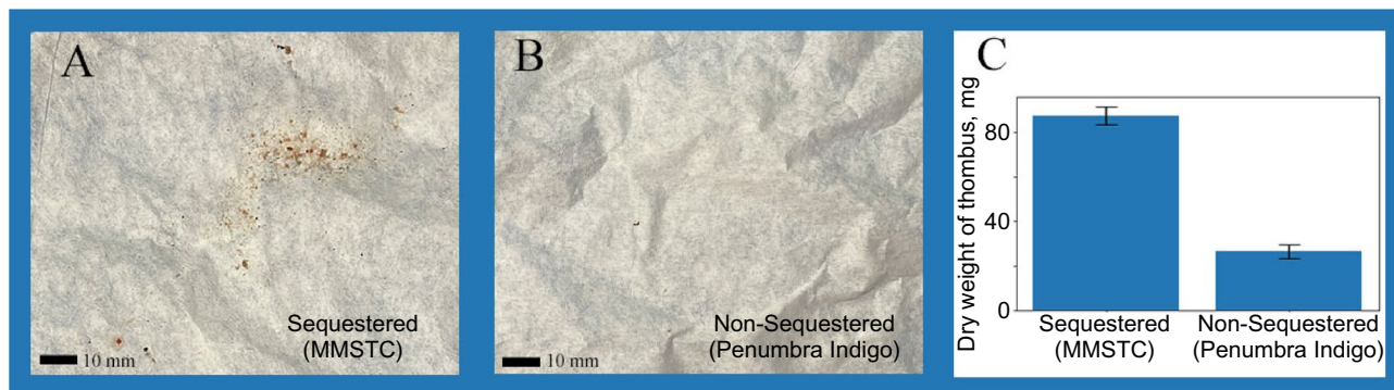
Figure 5. (A) Thrombus evacuated by the MMSTC in a typical experiment, viewed on filter paper, over the course of a 30 s treatment within the flow system. (B) Thrombus evacuated by the Penumbra Indigo CAT 5 Fr catheter in a typical experiment, viewed on filter paper, over the course of a 30 s treatment within the flow system. (C) The MMSTC evacuated significantly more thrombus than the Penumbra Indigo CAT 5 Fr catheter under these conditions ( p = 0.005 ).
