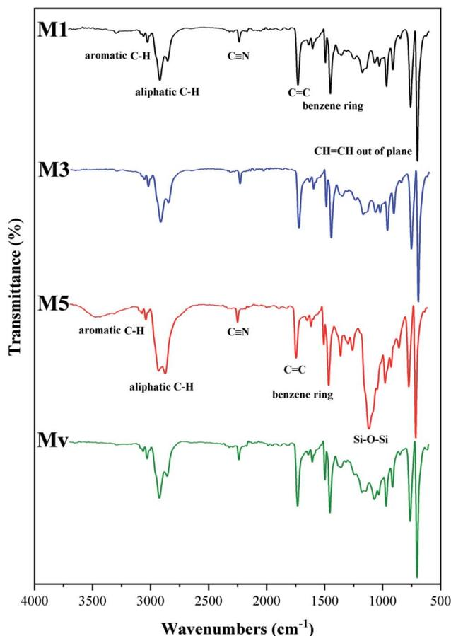
Fig. 7 ATR-FTIR spectra of neat and nanocomposite membranes.
