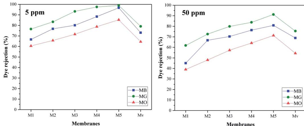
Fig. 15 Dye rejection of membranes at different concentrations.
