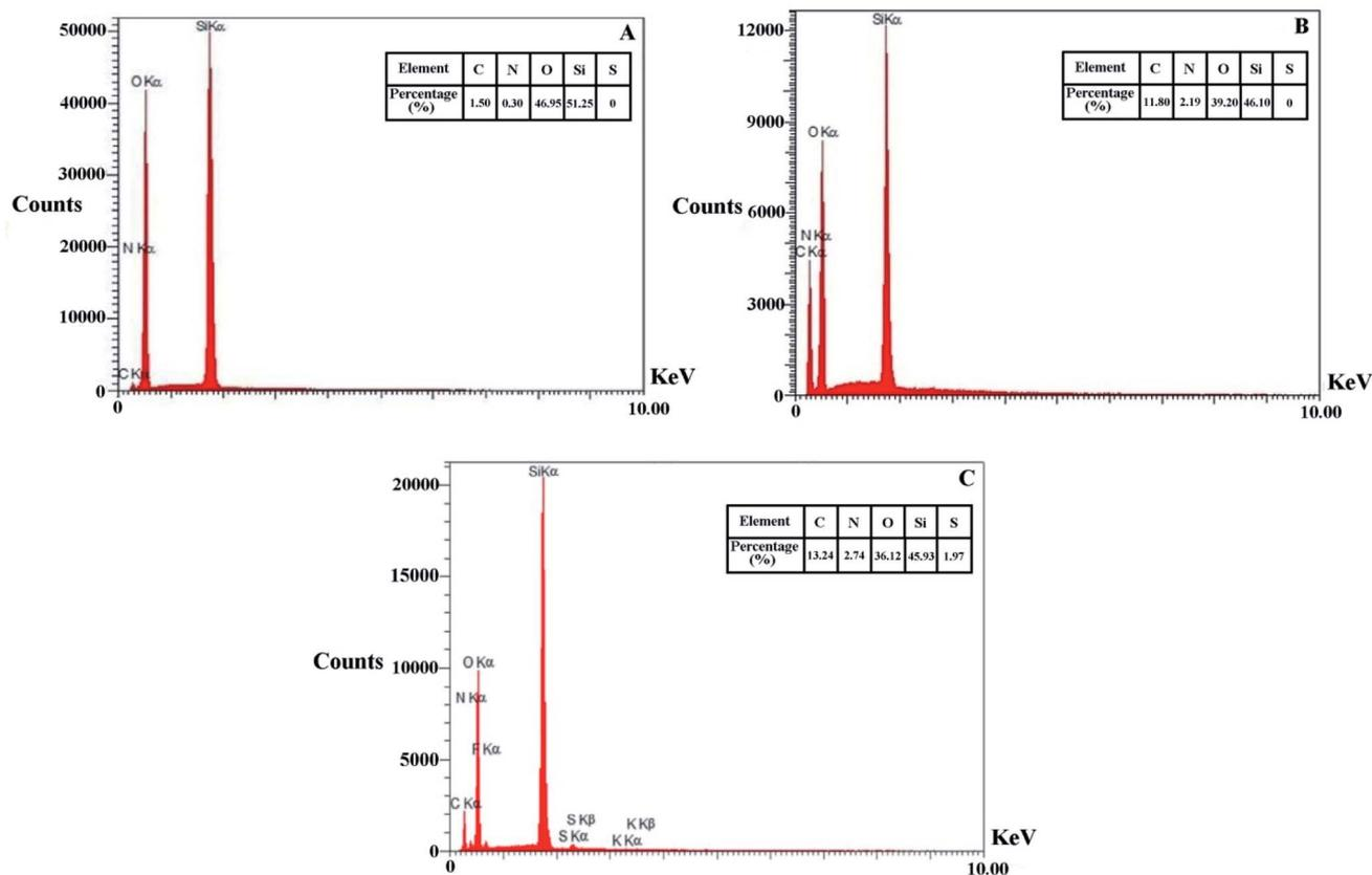
Fig. 4 EDAX elemental analysis of KCC-1, KCC-1-NH<sub>2</sub>, and KCC-1-NH-CS<sub>2</sub>.
