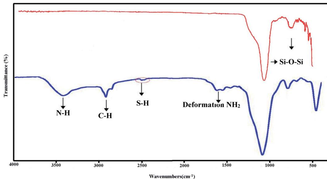
Fig. 2 FTIR spectra of KCC-1 and KCC-1-NH-CS<sub>2</sub>.
