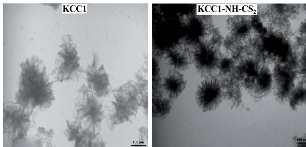
Fig. 3 FESEM and TEM images of KCC-1 and KCC-1-NH-CS<sub>2</sub>.
