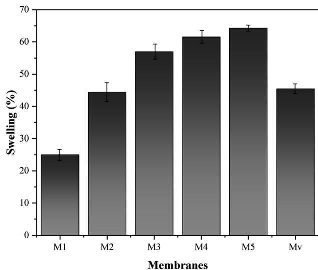
Fig. 10 Measured swelling for neat and nanocomposite membranes.
