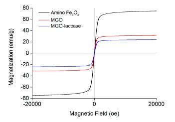
**Figure 2.** The magnetization curves of amino Fe<sub>3</sub>O<sub>4</sub> nanoparticles (**black**), MGO (**red**), and MGO-laccase (**blue**).
