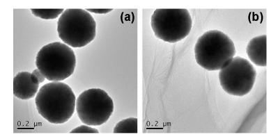
Figure 1. The TEM images of (a) amino Fe<sub>3</sub>O<sub>4</sub> nanoparticles and (b) MGO-laccase.
