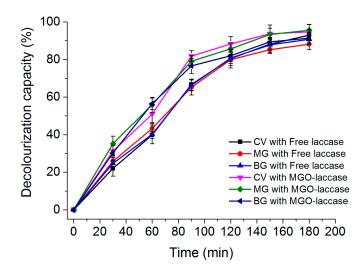
Figure 7. The removal rates of dyes (CV, MG, and BG) with free laccase and MGO-laccase.
