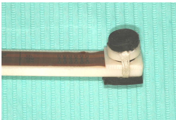
Figure 8 The pressure sensor with cushioned flexible pads to allow for accurate biting registration.
