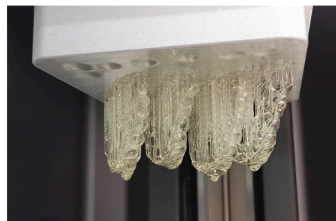
Fig. 5. Aligners printed in a vertical orientation. Note the supports that are needed for a successful printing which will be removed in the post printing procedure.
