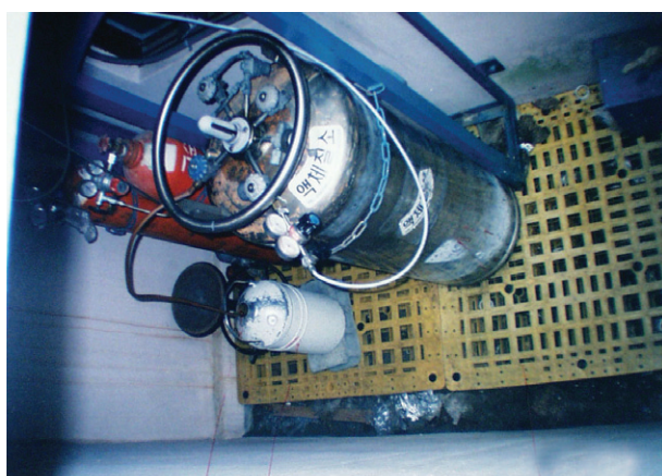
Fig. 1. The accident site in the underground dry area showed a LN 2 cylinder and a Dewar-flask that were linked to a copper tube in front of two O 2 tanks in a corner.
