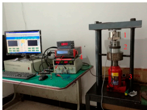
Figure 24. Experimental setup. (1) Particle damping sensor; (2) Standard sensor; (3) Hydraulic cylinder; (4) Displays.
