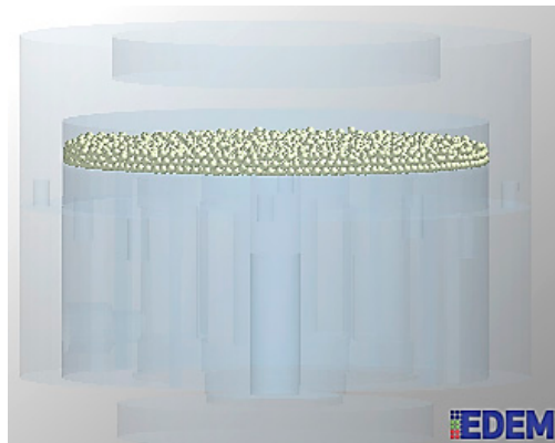
Figure 13. The model of particle damping sensor in EDEM.
