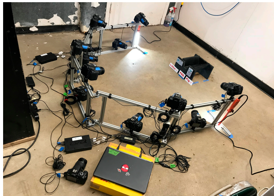
Figure 1. Photogrammetry rig and piglet cradle.
