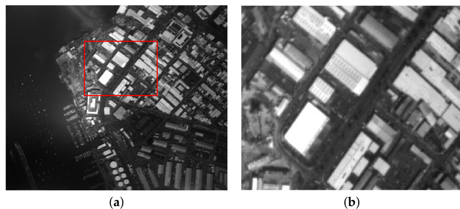
Figure 7. (a) Image taken with defocus; (b) enlarged view of the marked area.
