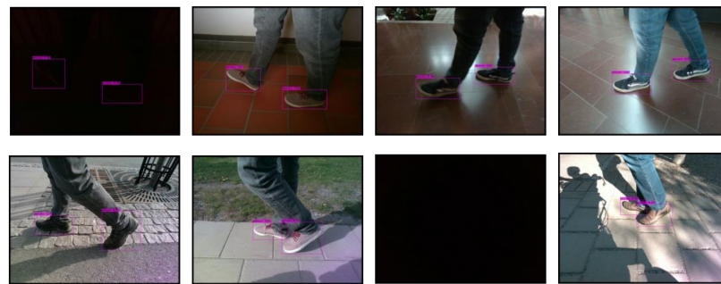
Figure 10. From top to bottom and left to right: YOLOv4-Tiny results using the 3-channel RGB frames for the 1-Indoor1-Dark, 2-Indoor1-Light, 3-Indoor2-Dark, 4-Indoor2-Light, 5-Outdoor1, 6-Outdoor2, 7-Darkness and 8-Outdoor5 scenarios.
