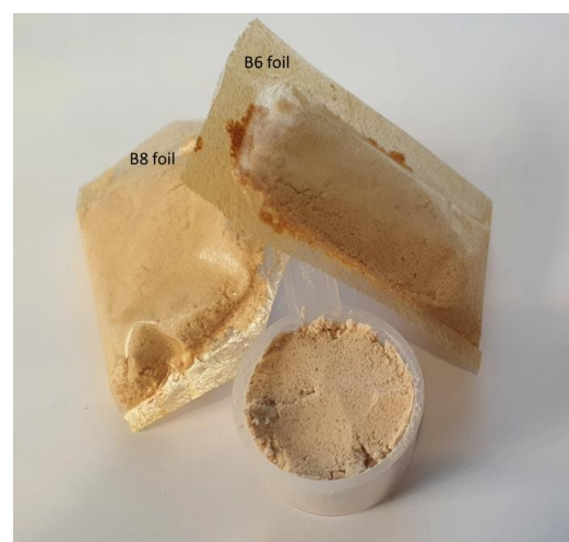
Figure 3. Examples of potential applications of developed films: protein powder packed in biopolymeric foils with orange (B6) and cinnamon (B8) EO added. Each package contains a measure of protein powder, according to the manufacturer. The packages are glued by hot thermowelding (180 °C, 20 s). The addition of orange and cinnamon EO may improve the sensorial properties of such powders and may sustain beneficial effect on health.
