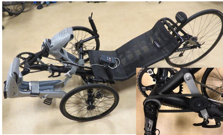
Fig. 1 Picture of the modified trike with ECU on the seat. Note the ankle immobilizers were utilized to lock out the ankle. The insert illustrates the gear on the crank arm which is attached to the encoder that provides crank position to the ECU
