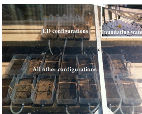
Figure 1. Outdoor experimental set up for the bank sediment survival study, which is covered by a transparent Perspex sheet; ED configurations placed on a higher platform and all the others on the lower platforms. Bottles containing water for inundating sediments (see upper right corner) were located on a vertically moving platform.
