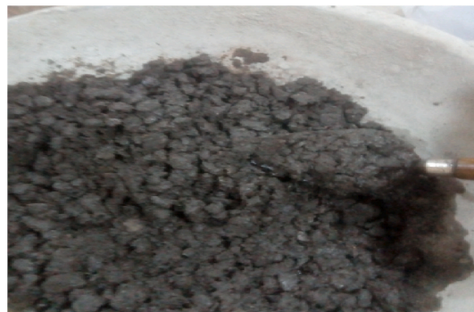
Fig. 2. Geopolymer concrete fresh mix.
