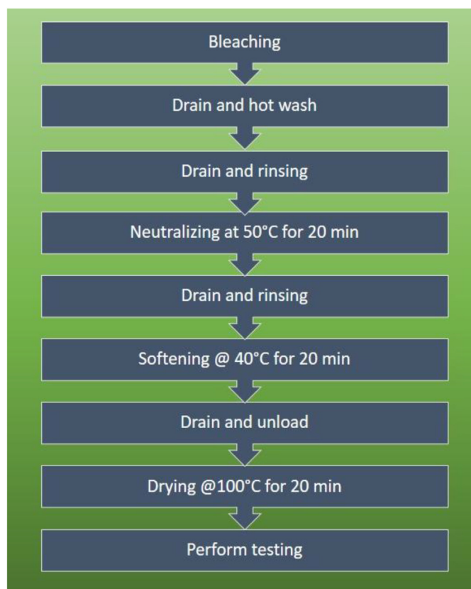
Figure 1. Process Sequence of Phenolic Yellowing treatment.
