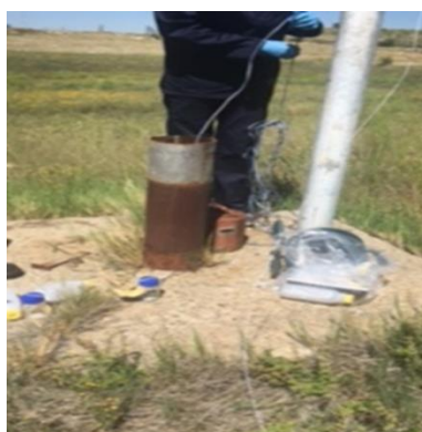
Figure 9. Well-constructed borehole in the northern landfill site.
