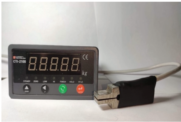
Figure 1. Bite force meter manufactured by the research team at the University of Medicine and Pharmacy, Ho Chi Minh City.
