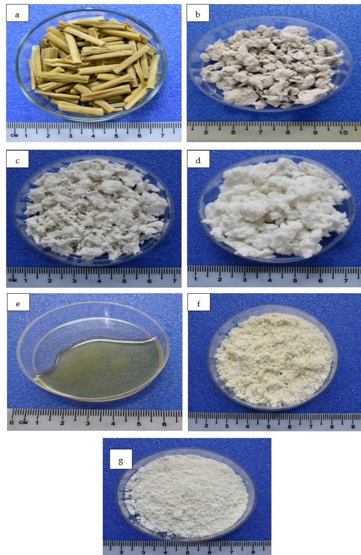
Figure 2. Photographs of (a) RS chip, (b) unbleached cellulose pulp (UPULP), (c) bleached cellulose pulp (PULP), (d) modified cellulose pulp (MPULP), (e) dissolve cellulose (DC), (f) cellulose powder (CP), and (g) modified cellulose powder (MCP).
