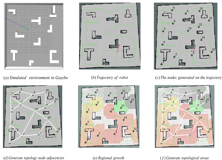
Figure 11. The topological map construction process in a similar environment (basically the same as the process in Figure 3). (a) is the simulated environment in Gazebo, (b) is the trajectory of robot, (c) is the nodes generated on the trajectory, (d) is the adjacency, (e) is the region dynamic growth algorithm and (f) is the Generated topological area.
