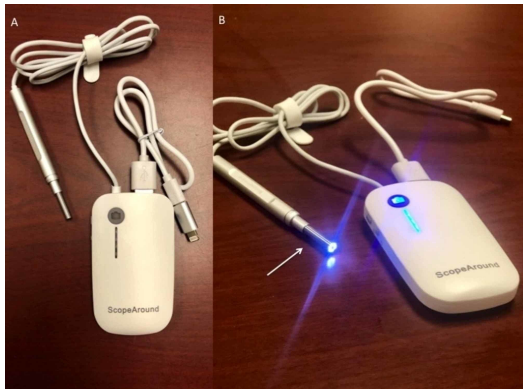
FIGURE 1: Video otoscope tool with attachable cord for smart device.
