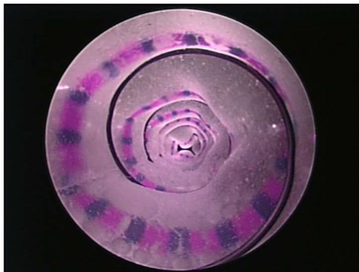
Fig. 8. Measurement of phantom cross-sectional area using telescope images.
