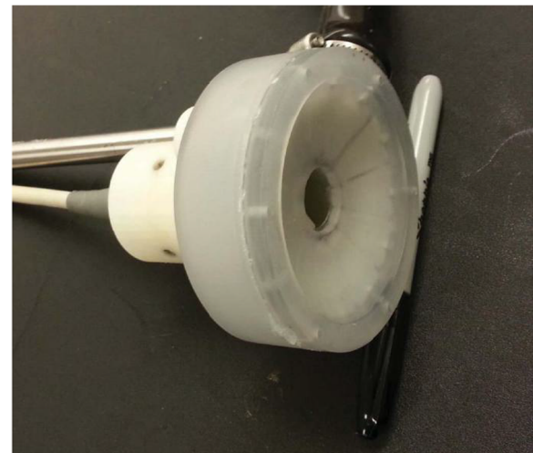
Fig. 77 (abstract O58). 12-element 1.5 MHz HIFU sector array transducer integrated with an ultrasound imaging probe (ATL P7-4)
