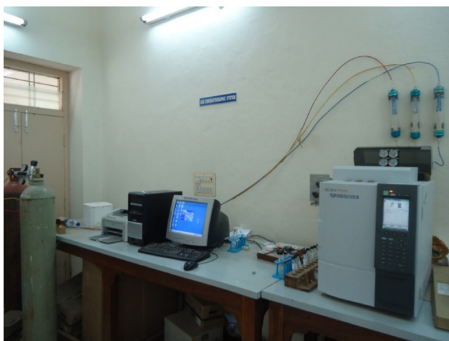
Fig. 2. The laboratory Gas Chromatography instrument for the analysis of the chemical components.
