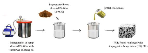
Figure 2. Synthesis of PUR foams reinforced with HS fillers.
