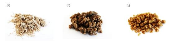
**Figure 1.** Hemp shives (HS) fillers used as reinforcing fillers: (**a**) non-treated hemp shives (HS), (**b**) hemp shives impregnated with sunflower oil (HS/SO), and (**c**) hemp shives impregnated with tung oil (HS/TO).
