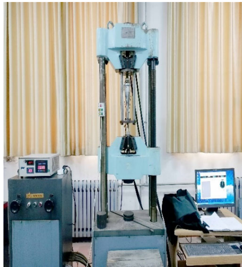
Figure 13. Schematic of the ultrasonic vibration tensile device.
