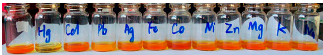
Figure 9. The response of coordination compound Ir1 acetonitrile solution to various metal ions ( \text{Hg}^{2+} , \text{Cd}^{2+} , \text{Pb}^{2+} , \text{Ag}^+ , \text{Fe}^{2+} , \text{Co}^{2+} , \text{Ni}^{2+} , \text{Zn}^{2+} , \text{Mg}^{2+} , \text{Na}^+ and \text{K}^+ ).
