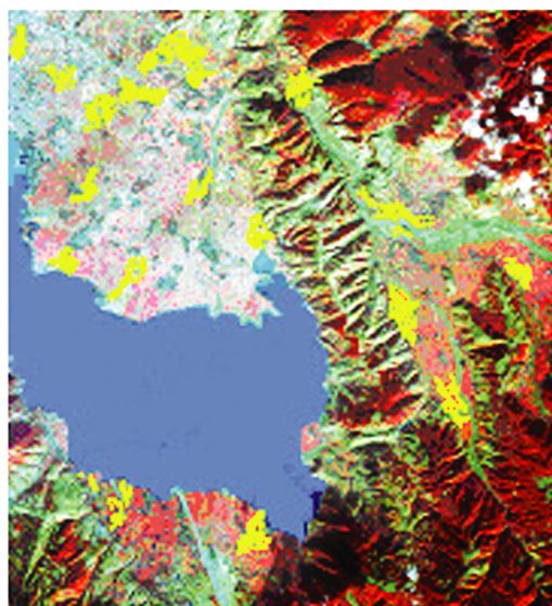
Fig. 3. The IKONOS image of Xichang acquired in December of 2000. The false color image is made from a combination of green, red and near infrared bands displayed with a color gun of blue, green and red, respectively. The yellow areas are the ditches where field snail surveys were conducted in 19 villages.
