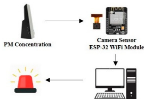
Figure 5. Overview of the data communication module system.
