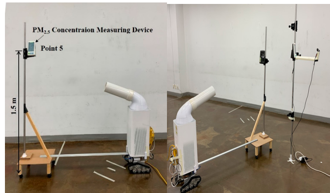
Figure 10. A method of implementing the air purifier that tracks occupants in real-time.
