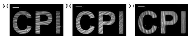
Figure 4. Fluorescence microscope images of microstructures produced with PDMAA- co -AOQ- co -RAS on (a) PMMA (polymeric substrate), (b) glass slide (inorganic substrate), and (c) gelatin (biomaterial-based substrate). Scale bars: 200 \mu\text{m} .
