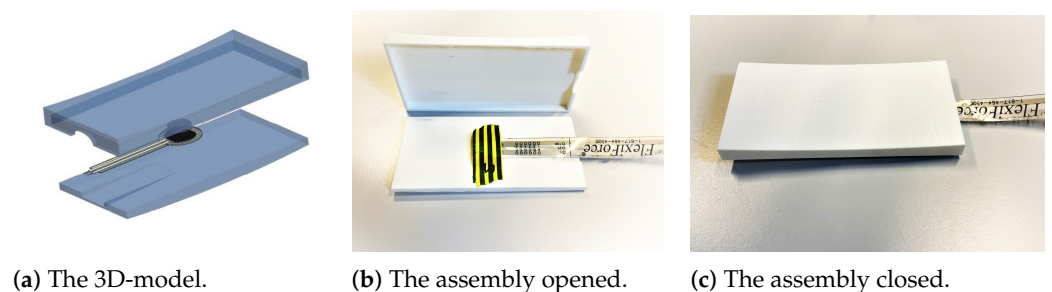
Figure 3. The 3D-model and the printed model of the concave shape, assembled with the sensors.
