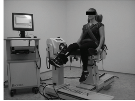
FIGURE 2: Test stand for the measurement of muscle torque.
