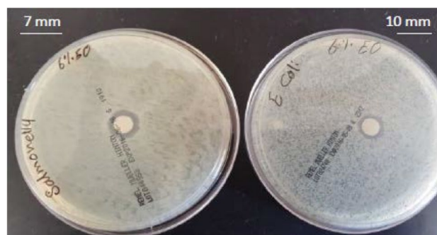
Fig. 7 Antimicrobial activity through inhibition zones of starch-MMT-6% v/v thyme essential oil bionanocomposite against E. coli and S. typhimurium [70]
