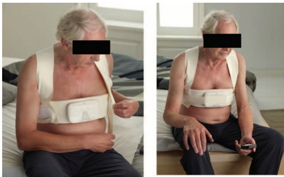
Figure 1 Bio-impedance monitor consisting of an adjustable vest with integrated textile electrodes and a slim electronics case.
