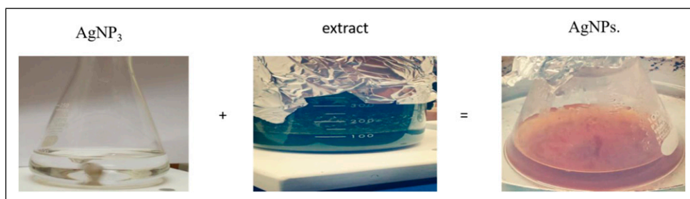
Figure 2. Synthesis of silver nanoparticles using M. oleifera leaves extract.
