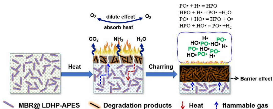
Scheme 2. Depiction of the flame retardant and smoke suppression mechanisms exhibited by MBR@LDHP-APES in EP.
