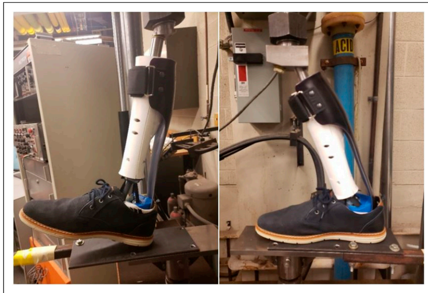
Figure 13. SLL-AFO attached to Instron in heel position (left) and forefoot position (right).
