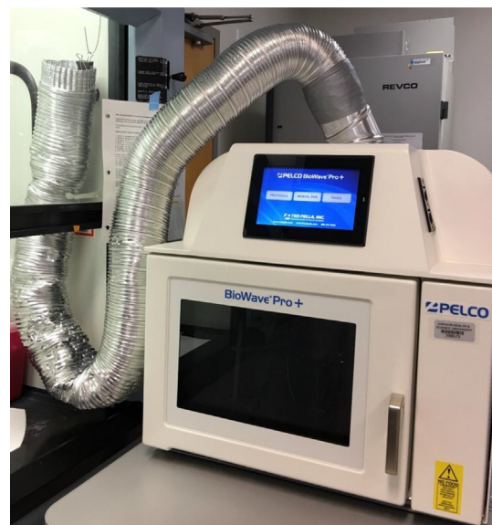
Figure 1. Microwave Pro + arrangement near the chemical hood. Notice that the exhaust is vented into the chemical hood.
