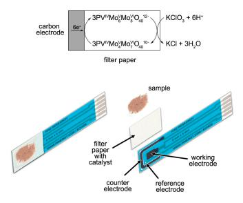
Scheme 1. Paper-based electrochemical detection of chlorate.
