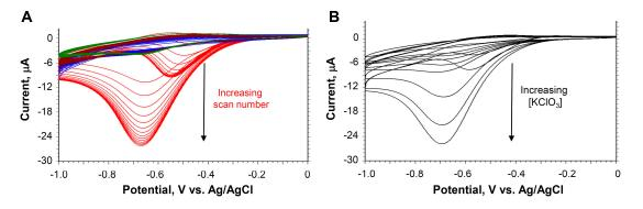
**Figure 1.** (**A**) Cyclic voltammograms with increasing scan number at 100 mV/s for the paper-based electrochemical probe containing 0.05 mg  $[PMo_{11}VO_{40}]^{5-}$  in 100 µL of buffer. Background (blue), NaNO<sub>3</sub> (brown), KNO<sub>3</sub> (green), KClO<sub>3</sub> (red) all at 5 mg/mL. (**B**) Cyclic voltammograms with increasing [KClO<sub>3</sub>]from 0.078 to 5 mg/mL.
