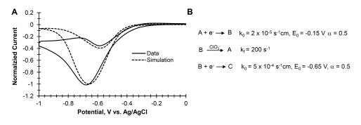
**Figure 7.** (**A**) Baseline subtracted cyclic voltammogram (solid line) at  $[KClO_3] = 5 \text{ mg/mL}$  compared to the simulated model (dotted line). (**B**) The electrochemical model used in the digital simulation.
