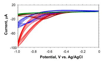
**Figure 2.** Cyclic voltammograms for the paper-based electrochemical probe in 100  $\mu$ L of buffer containing 0.05 mg (green) of [PMo<sub>11</sub>VO<sub>40</sub>]<sup>5–</sup> and with 5 mg/mL of KClO<sub>3</sub> (brown) or 0.4 mg of [PMo<sub>11</sub>VO<sub>40</sub>]<sup>5–</sup> (blue) and with 5 mg/mL of KClO<sub>3</sub> (red).
