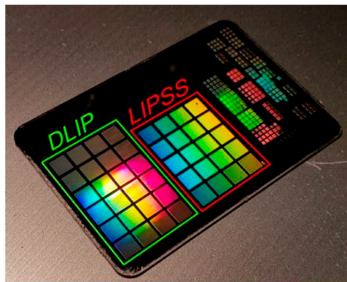
Figure 7. Photograph of structural colors generated on a polished steel plate by DLIP and LIPSS processing, as indicated on the sample. Reproduced from Soldera et al. [50], with permission from Japan Laser Processing Society.
