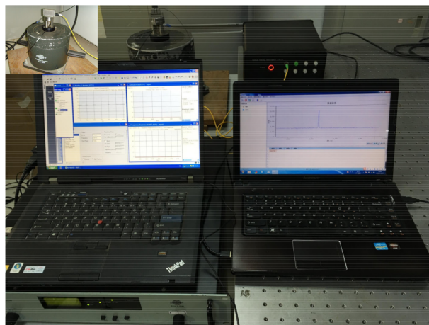
Figure 18. Accelerometer dynamic calibration testing system.
